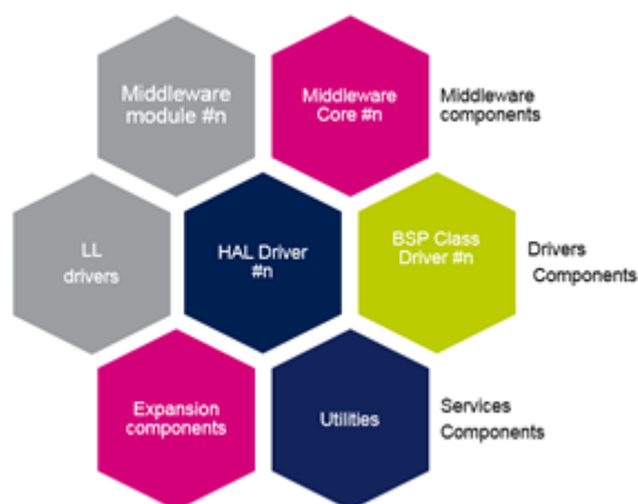
Figure 15. STM32Cube firmware components
