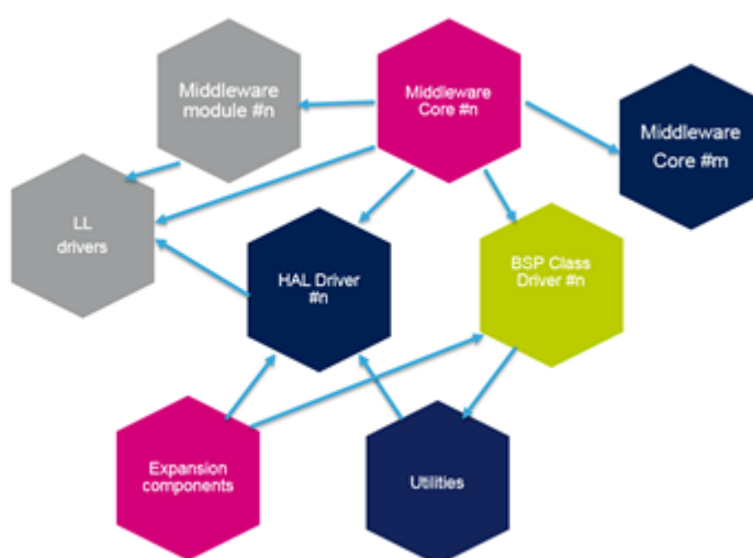
Figure 16. STM32Cube firmware component interactions
